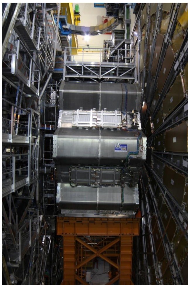
Ultra-wide-angle photo (14 mm lens) of our view into ATLAS, with muon detectors on either side. The main body of ATLAS containing the calorimeters and solenoid magnets is some 20 meters to the left.
