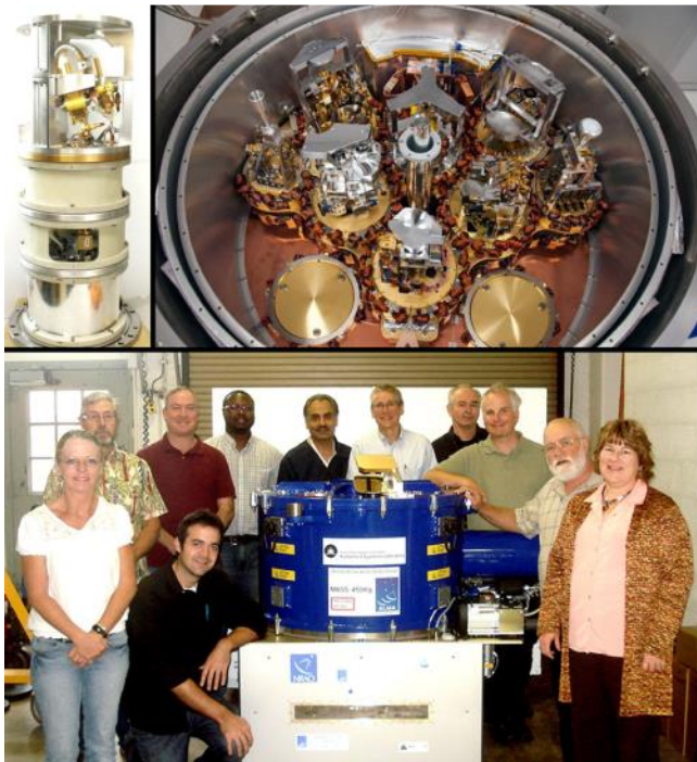
One of the receiver cartridges (upper left), the inside a cryostat with all 10 receivers in place (upper right) and the team from the Rutherford Appleton Laboratory (UK) that assembled the first cryostat in 2009 (ALMA)
