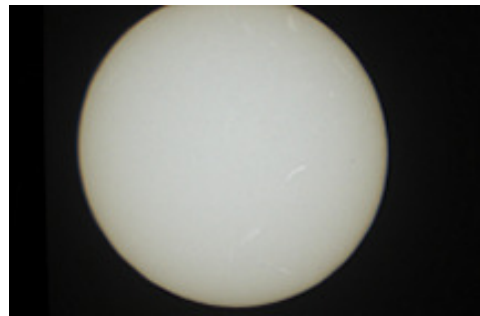
◀ John Paladini, trying to reproduce telescopes of old, ground a lens using 1/4-inch-thick window glass. The lens is 5 inches in diameter, but masked down to increase f/ratio and reduce aberrations. ▼ Projected image of the Sun focuses 24.5 feet from lens. Photos: John Paladini.
