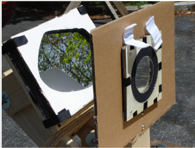
◀ John Paladini, trying to reproduce telescopes of old, ground a lens using 1/4-inch-thick window glass. The lens is 5 inches in diameter, but masked down to increase f/ratio and reduce aberrations. ▼ Projected image of the Sun focuses 24.5 feet from lens. Photos: John Paladini.
