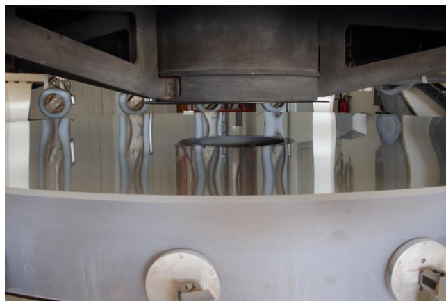
3.58 meter NTT mirror showing some of the lateral actuators and the central perforation
