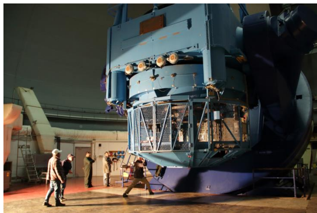
Another view of the primary case and horseshoe polar mount of the 3.6-meter telescope.
