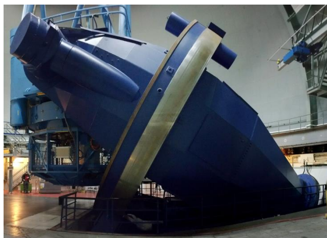
Polar drive bearing (silver ring) on the horseshoe mount
