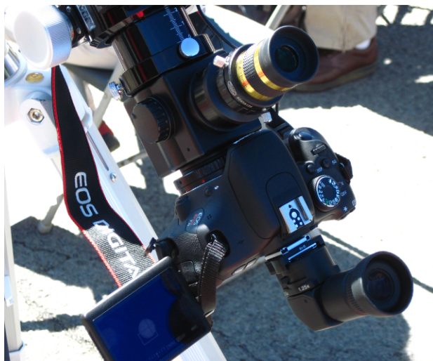
The business end of my setup: flip-mirror, 18 mm Plossl eyepiece on helical focuser, Canon T3i with angle finder
