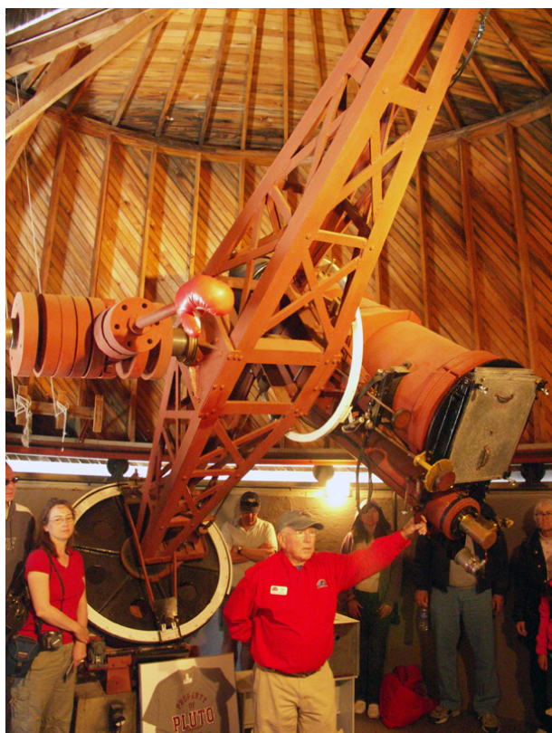
At the Pluto Discovery Telescope, a 13" refractor astrograph
