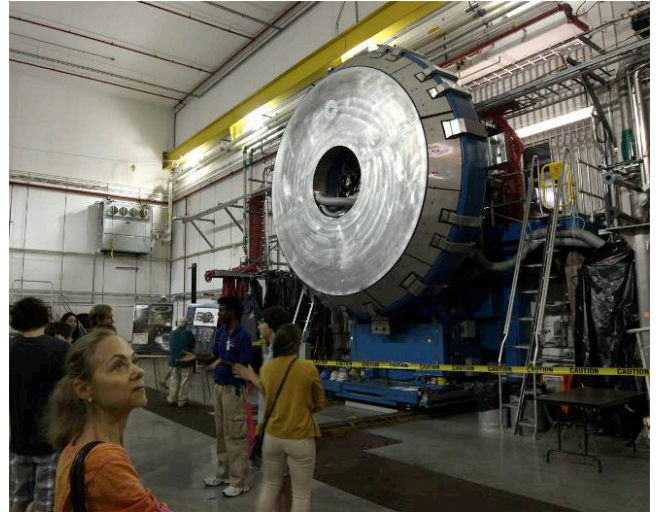
One beam portal at STAR. The device is rolled back into position and the Time Projection Chamber mates with this housing. There's one on the other side. (LF)
