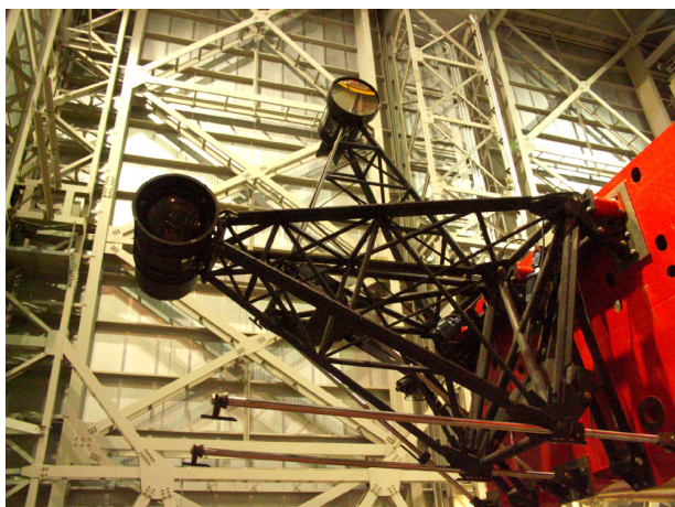
Prime focus camera (left) and secondary mirror (above) on their swing arms
