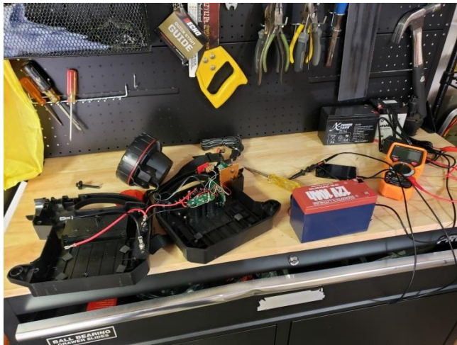
The old PowerTank opened, with the replacement battery on the right.
