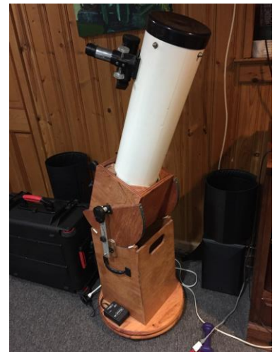
Parks Optical 6” f/8 Newtonian on home-made mount with encoders and Nexus II DSC
