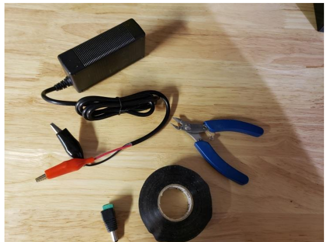
The charger with its alligator clips and the replacement male connector ready to installation.
