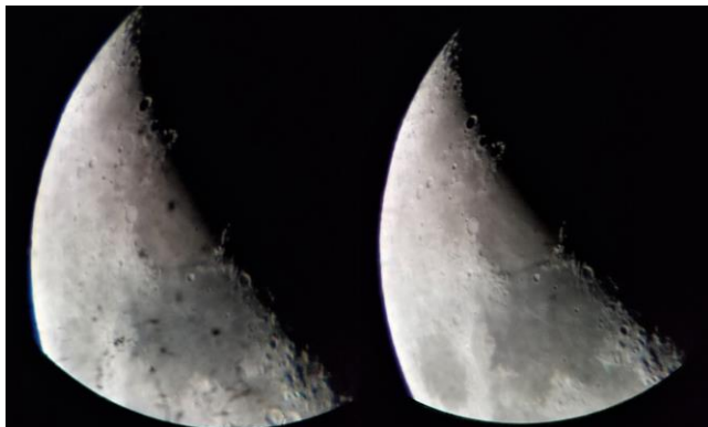
(L) Dirty eyepiece, (R) Clean eyepiece
