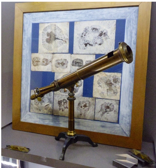
One of Secchi's spectroscopes and his drawings of sunspots. Note the prisms at the lower right corner of the image (LF)
