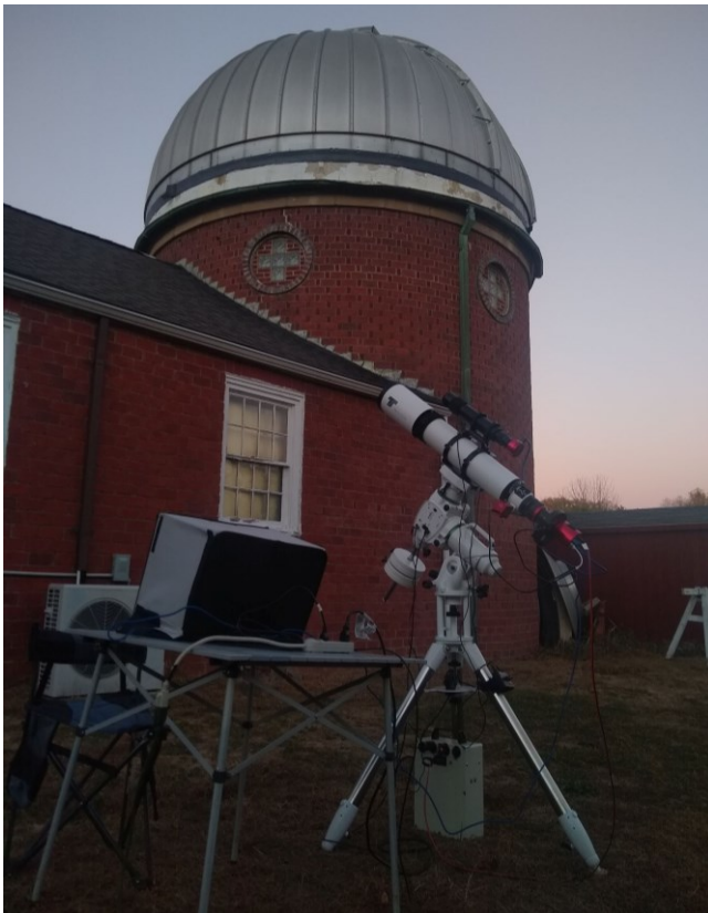
Steve’s set-up at Custer Institute. The scope is a TSO-115mm triplet f/7 refractor with a TSO 1.0X field flattener. An ASI294MM camera was used with narrowband filters.
